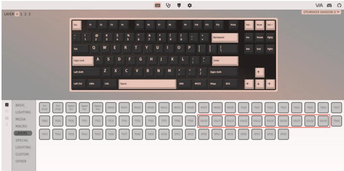
For instance, if you configure the Fn key on Layer 0 to OSL(2) and assign the Z key on Layer 2 to input the number 3, pressing the Fn (OSL(2)) key briefly, followed by the Z (3) key, will result in the input of the number 3. Thus, the OSL function enables a temporary switch to Layer n with a brief key press, and after a key on Layer n is triggered, it seamlessly returns to Layer 0.
