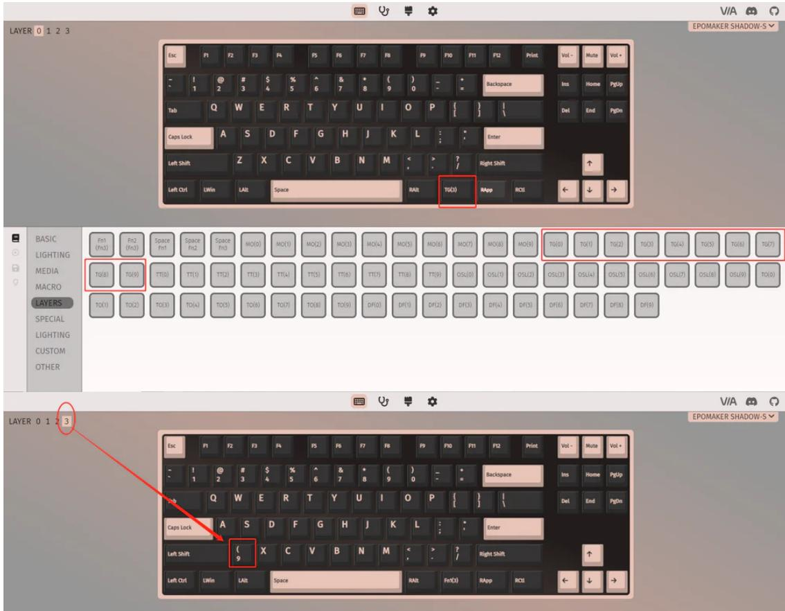
Once the keyboard is permanently switched to Layer 3 using TG(3), it remains on this layer until manually switched back. To return to Layer 0, you can employ one of the following methods:
