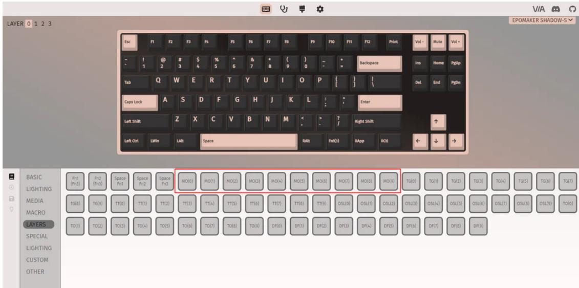
For example, if I set the Fn key on Layer 0 to MO(1) and assign the Z key on Layer 1 to the number 1, pressing and holding the Fn (MO1) key while pressing the Z (1) key will result in the input of the number 1, reverting to the base layer once the key is released.
